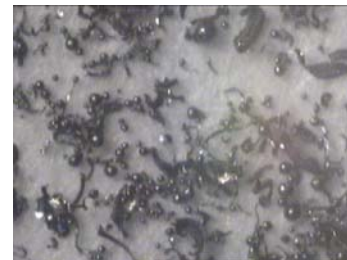
Fig 10. Chips obtained under dry grinding
