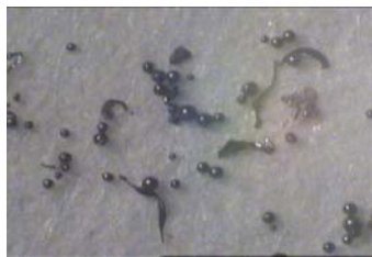
Fig 13. Chips obtained under ice cooled compressed air condition
